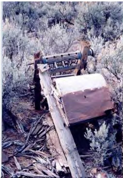
Figure 1 Left: A threshing machine for beans or triadora at the old homestead of Luis Trujillo (Photo courtesy of Chris Chávez c. 1998). Right: A hypothetical rendering of how the hand built machine may have operated (Illustration by Roberto H. Valdez).
